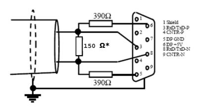
NOTE: Inversion of the two wires is not allowed! \* 150  $\Omega$  is the available value for line Type and B
